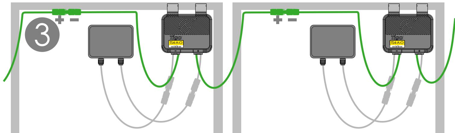
Note: When installing TS4-A, connect the input cables to the PV module before connecting the TS4-A output cables in series.
